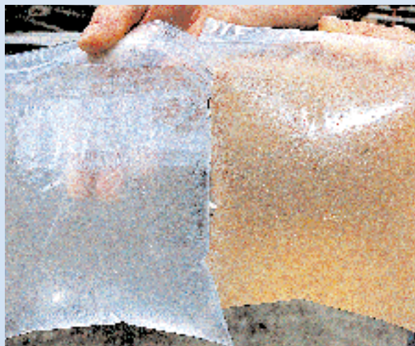
Figure 2. Before (right) and after (left): the filtration and treatment with ozone of chiller water with the AWP system
